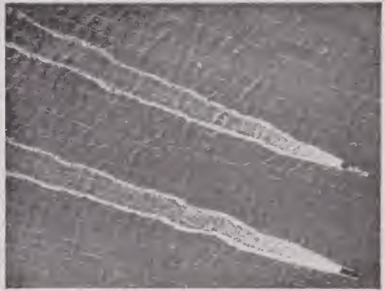
FIGURE 14. Effect of foam suppressor equipment on experimental DUKW (lower), in foamy, turbid water, Banana River, Florida.
